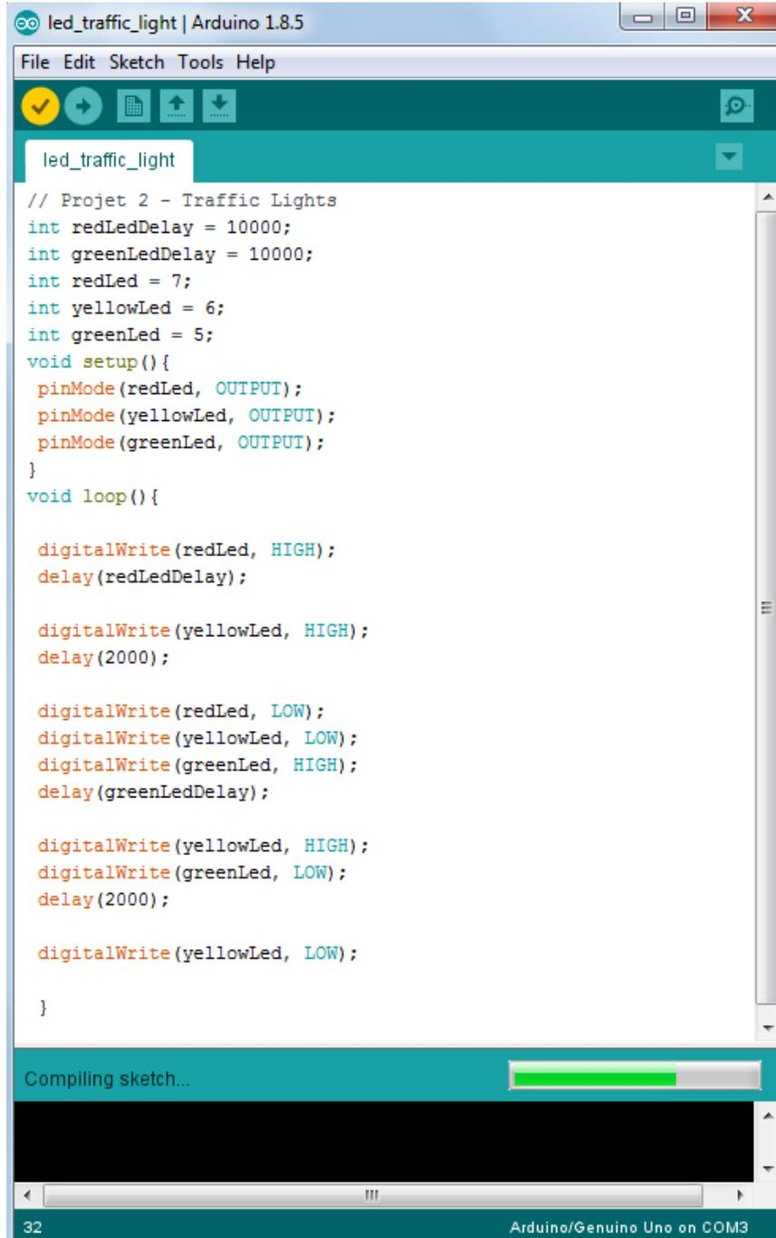
The screenshot shows the Arduino IDE interface with the sketch 'led\_traffic\_light' open. The code is as follows:
