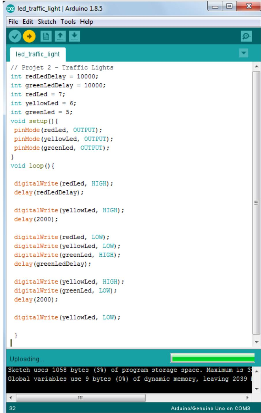
The screenshot shows the Arduino IDE interface with the sketch 'led\_traffic\_light' being uploaded to an Arduino/Genuino Uno board. The code in the editor is as follows:
