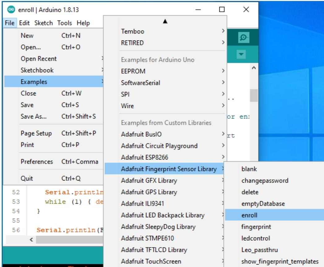
2. New windows of code will pop-out. Make sure correct Board type & port selected. Then **Upload** the code to Arduino. If using **Arduino MEGA** make sure to **change Pin**.
