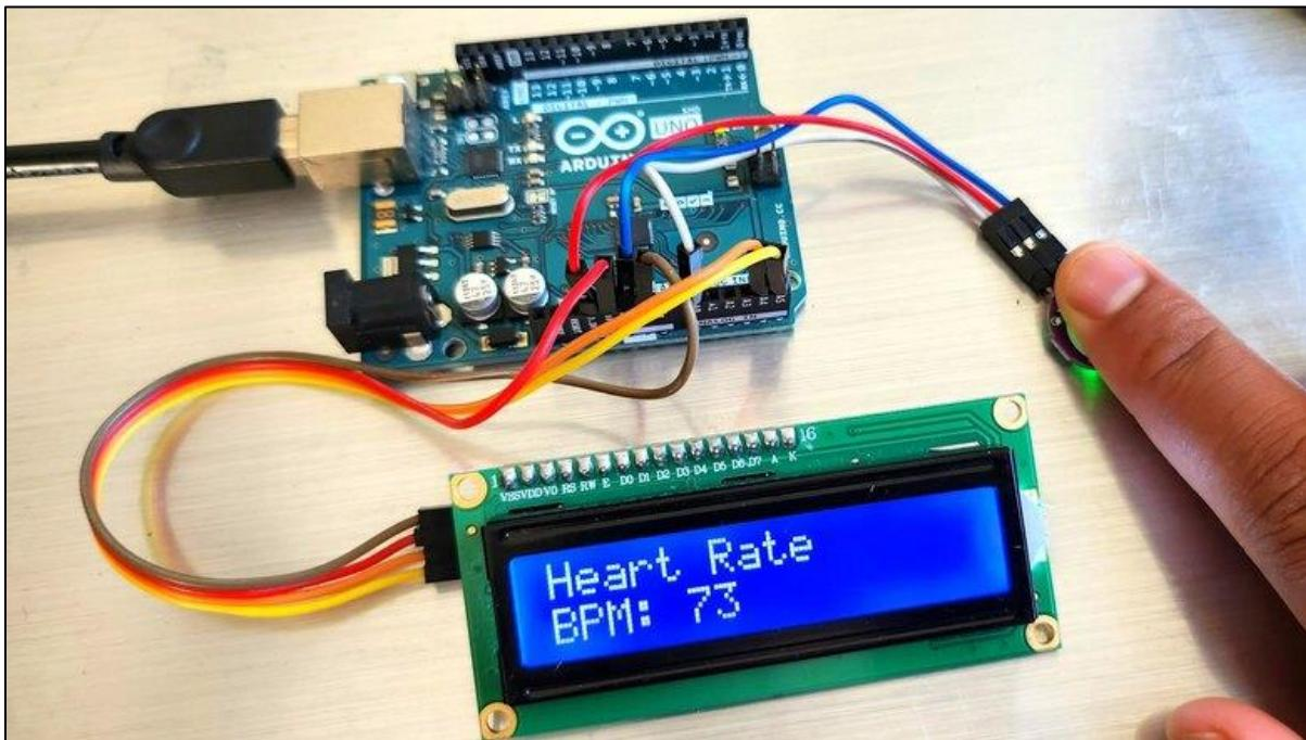
**Step 7:** After uploading the sketch, the readings may not be immediately accurate. To get reliable results, try to keep your finger as steady as possible while waiting.
