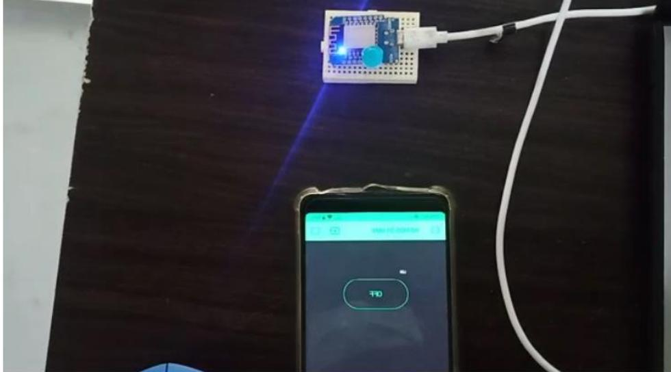
Once you upload the code successfully, green LED will start blinking if you switch the button ON. This tutorial was easy using Wemos D1 mini NodeMCU programming with simple steps.
