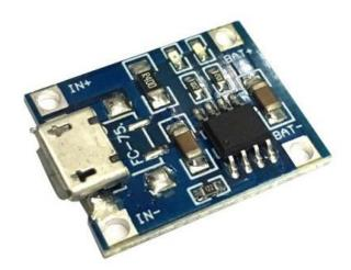
This charging board capable of charging single cell lithium batteries using the constant current to constant voltage charging method. The board on top adds additional circuitry which provides over-discharge, over current, and short circuit protection. It also uses a micro USB connection instead of mini USB. The boards feature two indicator LEDs, a green or blue LED to indicate that the battery is fully charged, and a red LED to indicate that the battery is charging.
