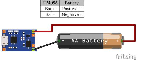
2. Connect the Micro USB cable and turn on the switch the Red indicator LED will light up means the battery still in charging condition.
