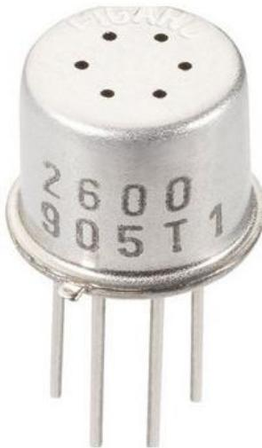
The sensing element is comprised of a metal oxide semiconductor layer formed on an alumina substrate of a sensing chip together with an integrated heater. In the presence of a detectable gas, the sensor's conductivity increases depending on the gas concentration in the air. A simple electrical circuit can convert the change in conductivity to an output signal which corresponds to the gas concentration.
