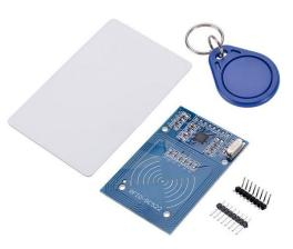
This RFID module is based on MFRC522 which is a highly integrated reader/writer IC for contactless communication at 13.56 MHz. It support Mifare family card and ISO14443 Type A card. RFID means radio-frequency identification. RFID uses electromagnetic fields to transfer data over short distances. RFID is useful to identify people, to make transactions and others. You can use an RFID system to open a door. For example, only the person with the right information on his card is allowed to enter.
