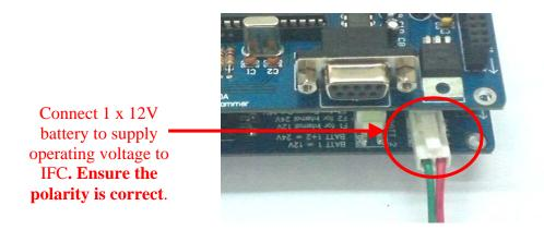
d. Turn ON the IFC power by pushing the toggle switch to "ON". There should be at least 3 LED (12V LED on Power Card, PWR LED on Main Brain and PWR LED on Control Panel) light up as shown.
