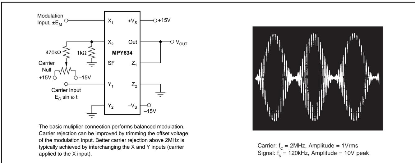
FIGURE 11. Balanced Modulator.
