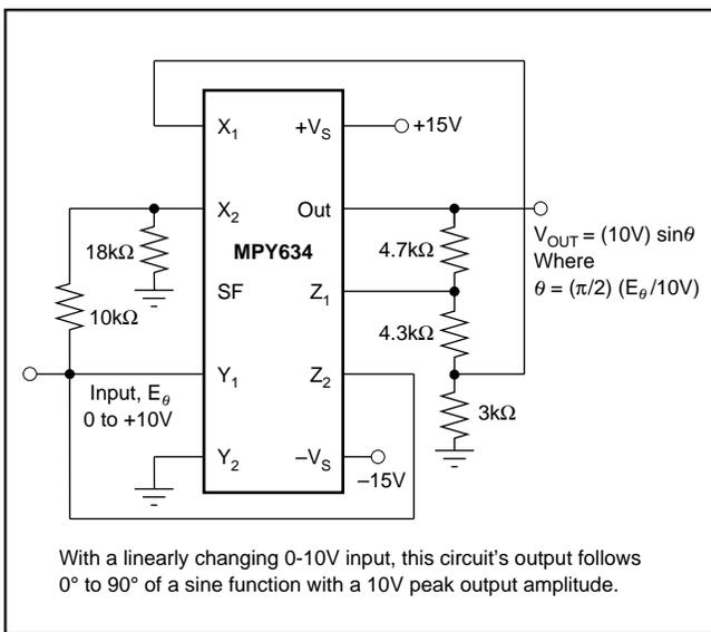
FIGURE 8. Sine-Function Generator.
