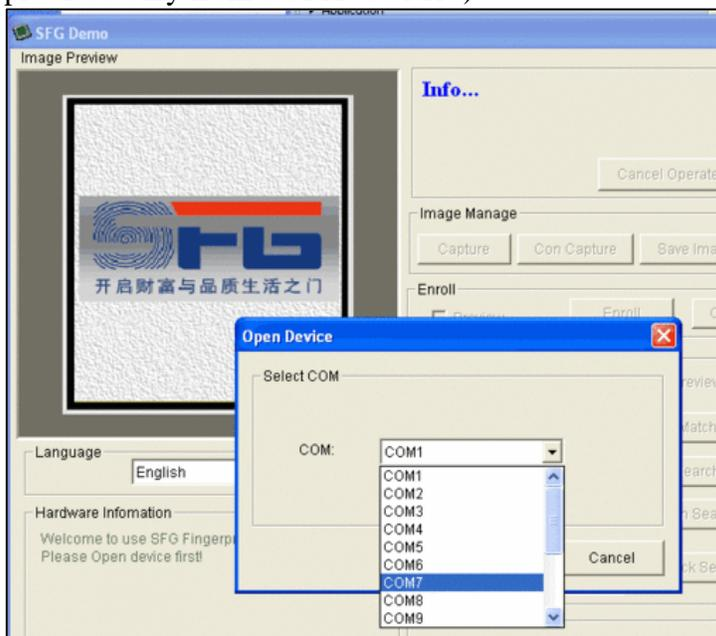
The software will show “Open Device Success” and “hardware information” on the screen. Then, change the baud rate and security level in the bottom left hand corner, as well as the "security level" (how sensitive it is). Set it to 57600 baud and security level 3.
