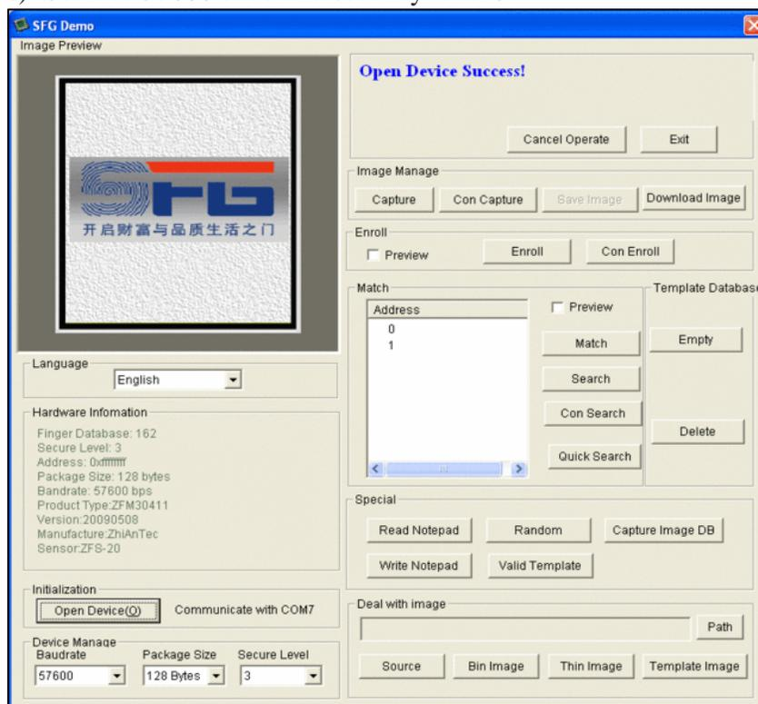
To enroll the new finger, click on the Preview checkbox and press the Enroll button. (Con Enroll means 'Continuous' enroll, which you may enroll for others fingerprint. When the box comes up, key in the ID by type “#” and followed by the number you desire. You can use up to 162 ID numbers.
