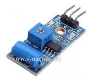
Vibration sensor is used originally as a vibration switch because of its high sensitivity. It is sensitive to environment vibration, and generally used to detect the ambient vibration strength. When the module does not reach the threshold in shock or vibration strength, DO port output goes high level and when external vibration strength exceeds the threshold, D0 port output goes low level.
