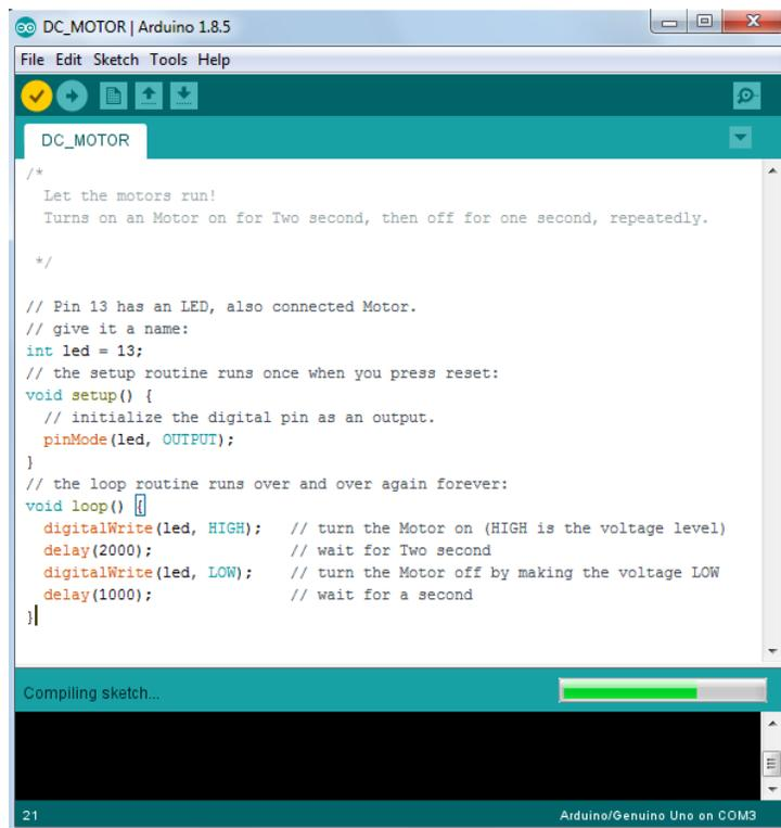
**STEP 4:** Upload the sketch to Arduino UNO. Click the Upload button. It will also turn orange and then blue once the sketch has finished uploading to your Arduino board.
