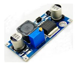
The LM2596 regulator is monolithic integrated circuit ideally suited for easy and convenient design of a step—down switching regulator (buck converter). It is capable of driving a 3.0 A load with excellent line and load regulation. This device is available in adjustable output version and it is internally compensated to minimize the number of external components to simplify the power supply design
