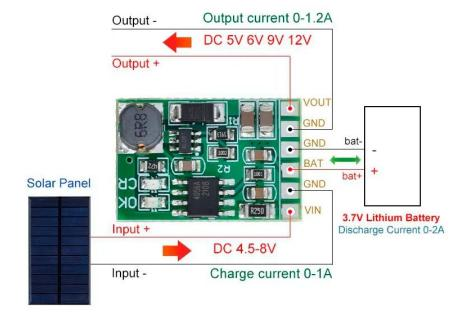
1. Connect the solar panel to the DC-DC Converter Boost Module, then connect the module to the lithium battery.
