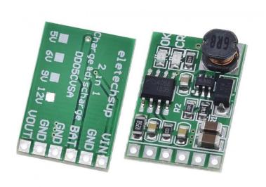
The DC-DC Converter Boost Module is a versatile 2-in-1 solution designed for solar mobile power applications. With support for both 5V and 12V output, this module efficiently charges and discharges lithium batteries. Its compact design and robust features make it an ideal choice for powering various devices in solar-powered setups, offering flexibility and reliability in renewable energy scenarios.
