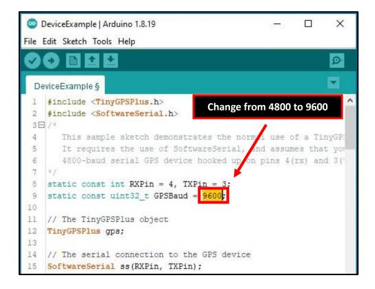
6. Once code correctly configured **Upload** the code to **Arduino UNO** board.
