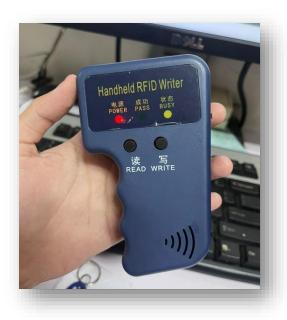
A 125kHz RFID re-writer is a specialized device designed for the manipulation of RFID tags operating at a frequency of 125kHz. Utilizing Radio-Frequency Identification (RFID) technology, this device serves as a crucial tool in the modification and retrieval of data stored on RFID tags. Comprising essential components such as a reader module, antenna, and microcontroller, the re-writer generates an electromagnetic field to communicate with and power passive RFID tags.
