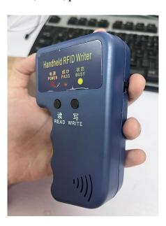
**Step 2:** Put the mother card near the antenna on the left side of the device, and then hit the READ button; the device will beep and the LED will turn on when the read is successful; if it beeps twice, move to step 3, and if it beeps three times, go to step 4. If it doesn't beep, click READ again.
