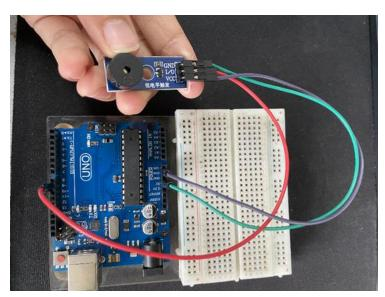
Step 2: Open Arduino IDE on PC and insert the given code below.
