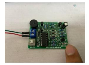
2. Mecury switch will move and trigger the buzzer.
