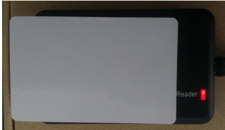
2. On **ID-RW-NO-Drive-EN** application / software click on **Connect** button. After the reader Status show '**Reader connection is successful**' check the **Analog USB Keyboard** option box. Next, click on Read Card the reader LED indicator should flashing.
