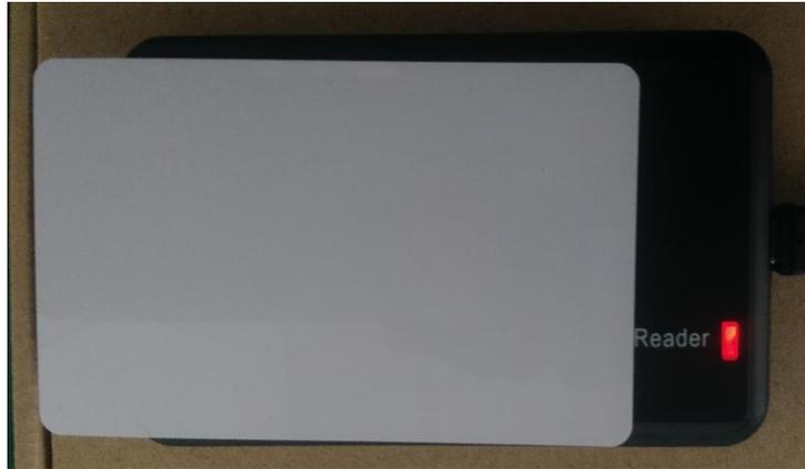
3. On **ID-RW-NO-Drive-EN** application / software click on **Connect** button. After the reader Status show '**Reader connection is successful**'. Fill in the 10H box with the new ID that want to be changed. Click on **Write Card** to start writing new value to Card.
