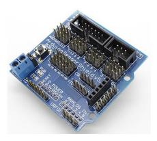
Arduino Controller Sensor Shield V5.0 allows you to connect to various modules like sensors, servos, relays, buttons and potentiometers. Each functional module has buckled port with VCC, GND and Output, which has corresponding port on the Sensor Shield, connected with a plain 2.54mm dual-female cable.
