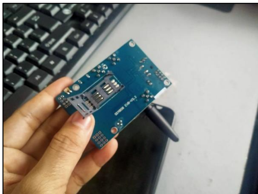
Pull up the SIM holder & then slide in the SIM card into the holder opening.
