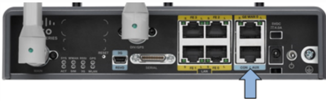
Figure 2. Example Console Port Labeled CONSOLE (Cisco 1811W Router)
