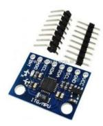
The MPU-6050 sensor module contains an accelerometer and a gyro in a single chip. It is very accurate, as it contains 16-bits analog to digital conversion hardware for each channel. Therefore it captures the x, y, and z channel at the same time. The sensor uses the I2C-bus to interface with the Arduino.
