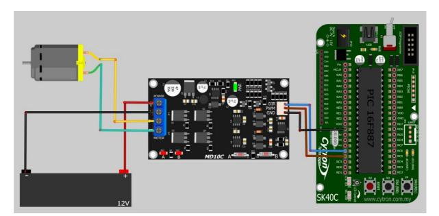
1. Connect MD10C and SK40C as shown in the schematic above and select the board supply for MD10C.
