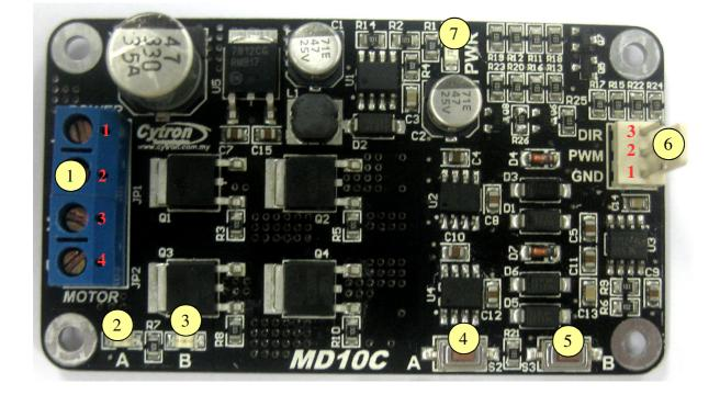
1. Terminal Block – Connect to motor and power source.
