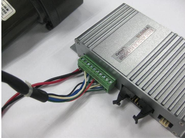
2. Connect power supply (thick red and black wire) to 24V power source.
