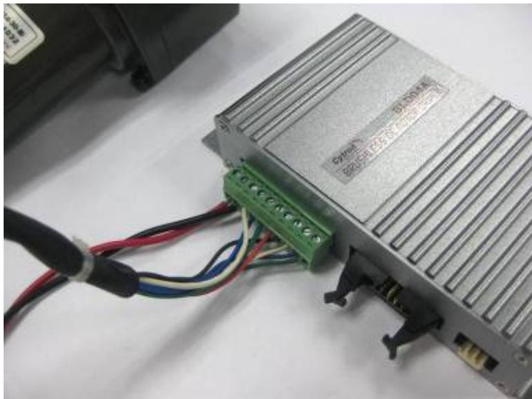
2. Connect power source wire (thick red and black wire) to 24V power source.
