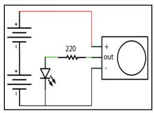
Now when the PIR detects motion, the Output pin will go "high" to and light up the LED. Once LED light up, wait for 10-60 seconds for the PIR to 'stabilize'. Wait until the LED is off and LED will light up when PIR detects motion in the infrared levels emitted by surrounding objects.
