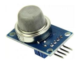
The MQ series of gas sensors use a small heater inside with an electro-chemical sensor. They are sensitive for a range of gasses and are used indoors at room temperature. The output is an analog signal and can be read with an analog input of the Arduino.
