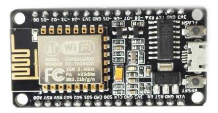
NodeMCU is a small board, based on the cheap ESP-12 Wi-Fi module containing a single-chip ESP8266 Wi-Fi SoC. The NodeMCU is an open-source firmware and development kit that helps you to prototype your IOT product within a few Lua script lines. The ESP-12 is one of the available modules containing an ESP8266 chip; it is becoming more and more popular because of its integrated Wi-Fi PCB antenna and shield.
