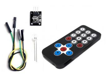
This Mini ultra-thin remote control has 17 function keys. Its transmit distances up to 8 meters, suitable for controlling indoor devices of all kinds. Infrared remote control receiving module can receive standard 38 KHZ modulation signals. The remote control signal decoding operation can be realized by programming the Arduino, which can be used in all kinds of remote control robots and interactive work.
