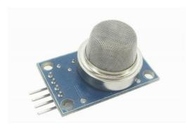
The MQ series of gas sensors use a small heater inside with an electro-chemical sensor. They are sensitive for a range of gasses and are used indoors at room temperature. The output is an analog signal and can be read with an analog input of the Arduino.
