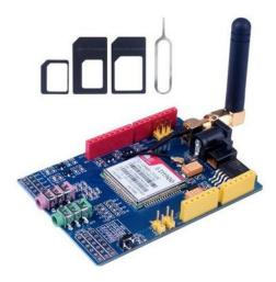
The GPRS Shield is based on SIM900 module from SIMCOM and compatible with all boards which have the same form factor (and pin-out) as a standard Arduino Board. The shield allows you to achieve SMS, MMS, GPRS and Audio via UART by sending AT commands (GSM 07.07, 07.05 and SIMCOM enhanced AT Commands). The shield also has the 12 GPIOs, 2 PWMs and an ADC of the SIM900 module (They are all 2V8 logic) present onboard.
