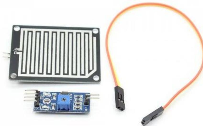
The rain sensor module is an easy tool for rain detection. It can be used as a switch when raindrop falls through the raining board and also for measuring rainfall intensity. It allows you to measure moisture via analog output pins and it provides a digital output when a threshold of moisture is exceeded.
