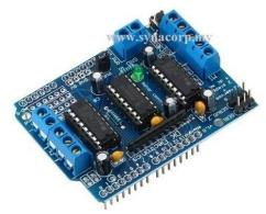
L293D is a monolithic integrated, high voltage, high current and 4-channel driver. This chip can drive DC motors with power supplier up to 36 Volts, and the chip also can supply a maximum current of 600mA per channel. L293D Dual Motor Shield has two L293D motor drivers and one 74HC595 shift register. The shift register expands 3 pins of the Arduino to 8 pins to control the direction for the motor drivers. The output enable of the L293D is directly connected to PWM outputs of the Arduino.
