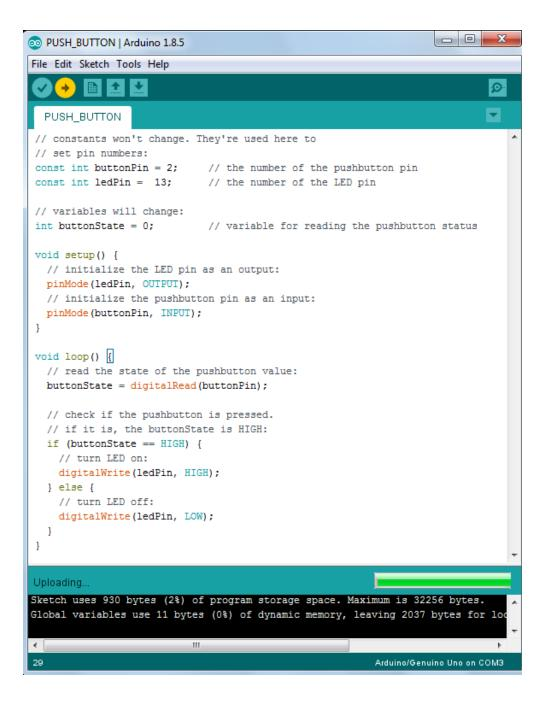
**RESULT:** When the pushbutton is open (unpressed) there is no connection between the two legs of the pushbutton, so the pin is connected to ground (through the pull-down resistor) and we read a LOW. When the button is closed (pressed), it makes a connection between its two legs, connecting the pin to 5 volts, so that we read a HIGH.
