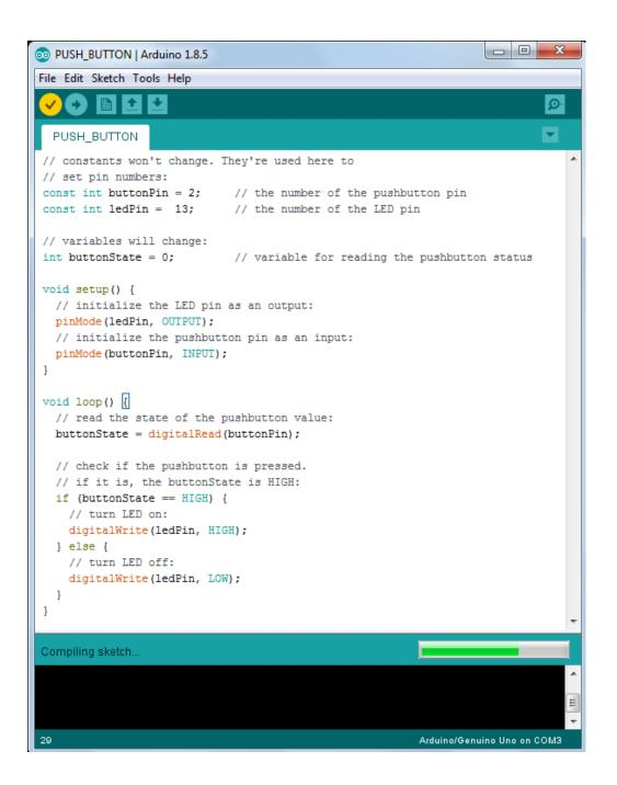
**STEP 4:** Upload the sketch to Arduino UNO board. Click the Upload button. It will also turn orange and then blue once the sketch has finished uploading to your Arduino board.
